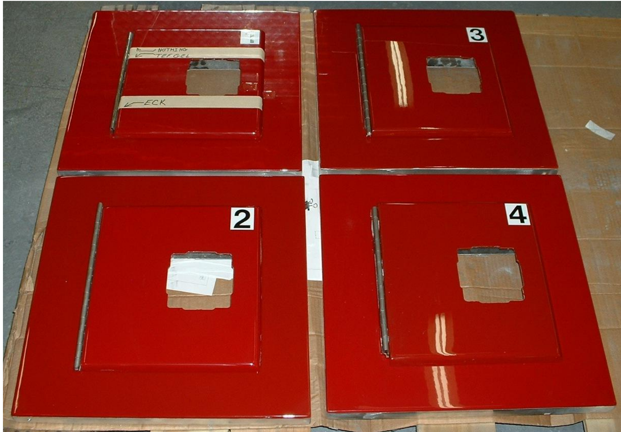
4 Test Panels – 1 st panel w/ nothing, Tef-Gel & ECK®, 2 nd panel w/ no protection, 3 rd panel w/ ECK® & 4 th panel w/ Tef-Gel.
